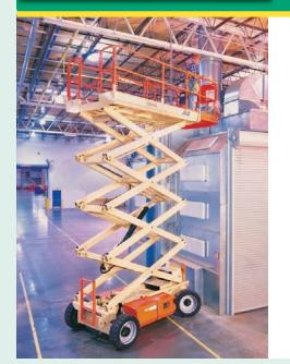
Working height 12.06m Working outreach 0.91m > Platform capacity 454kg Working width 1.75 1.75m x 3.10m > Width x length > Stowed height 2.74m
