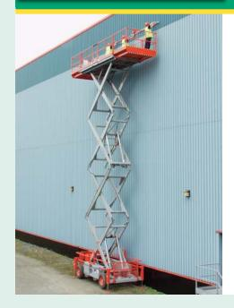
Working height 17.20m Working outreach 1.5m > Platform capacity 908kg Working width 2.34m > Width x length 2.34m x 4.50m > Stowed height 2.30m Weight 6,818kg 12 10 8
