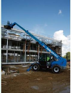
Working height 12.12m Max lift capacity 3500kg Max height lift capacity 2500kg Max reach lift capacity 1000kg Max forward reach 8.53m 1.17m › Reach at max height Weight 9,000kg
