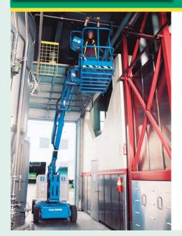
Working height 12.52m Working outreach 6.78m > Platform capacity 227kg > Working width 1.42m > Width x length 1.47m x 5.72m
