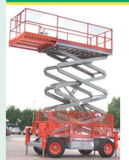
Working height 12.70m Working outreach 1.40m > Platform capacity 454kg Working width 1.60m > Width x length 1.82m x 3.30m > Stowed height 2.86m
