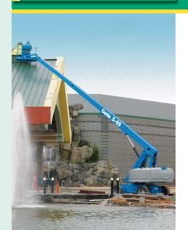
Working height 21.80m > Working outreach 17.10m > Platform capacity 227kg > Working width 2.44m > Width x length 2.49m x 9.50m
