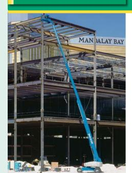
Working height 40.15m Working outreach 24.38m > Platform capacity 227kg Working width 2.44m > Width x length 3.35m x 14.25m
