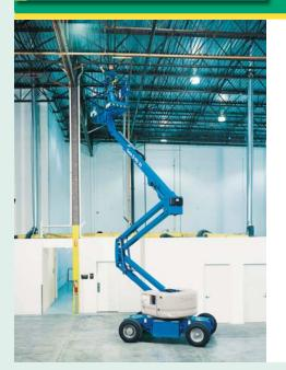
Working height 15.92m Working outreach 7.65m > Platform capacity 227kg > Working width 1.83m
