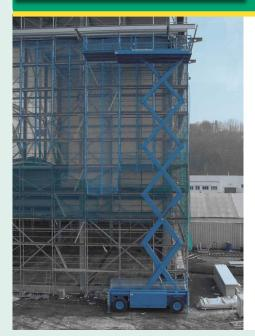
Working height 22.50m > Working outreach 2.20 > Platform capacity
